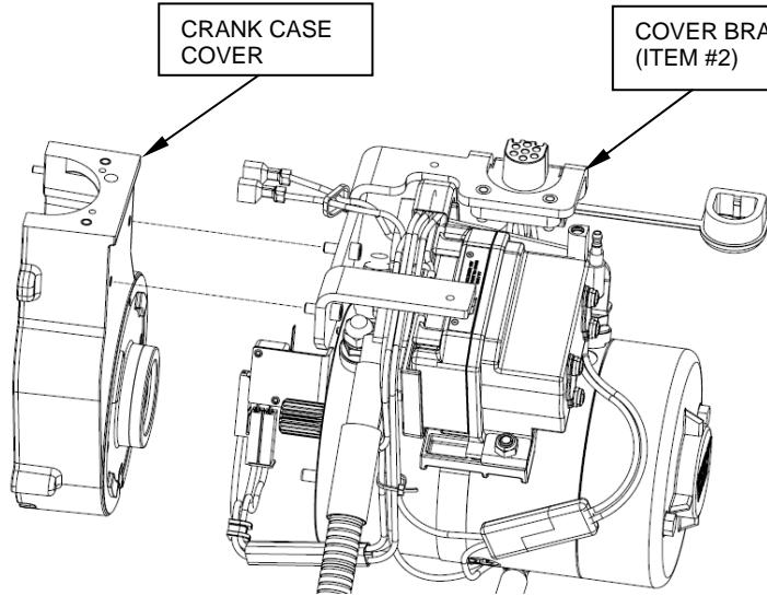
ATTACH MOTOR TO CRANK CASE HOUSING.
