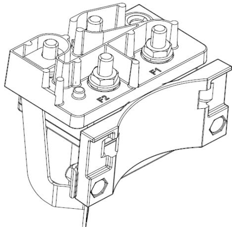
INSTALL SEPARATOR WITH BUS BAR ON CONTACTOR (ITEM #16)
