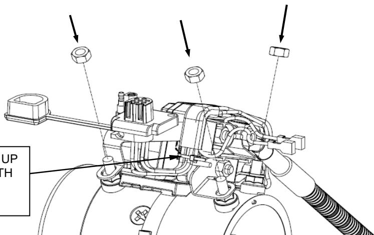
INSTALL CONTACTOR ASSEMBLY ON THE MOTOR. ATTACH THE CONTACTOR MOUNT (ITEM #7) TO THE MOTOR WITH HOSE CLAMP (ITEM #13).
