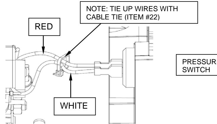
INSTALL HARNESS (ITEM #1) WIRES TO PRESSURE SWITCH AS SHOWN.
