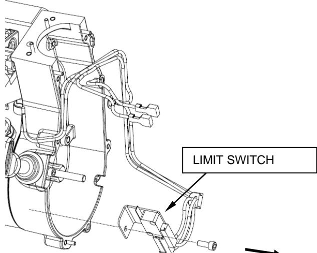
REMOVE LIMIT SWITCH INSIDE CRANK CASE COVER.
