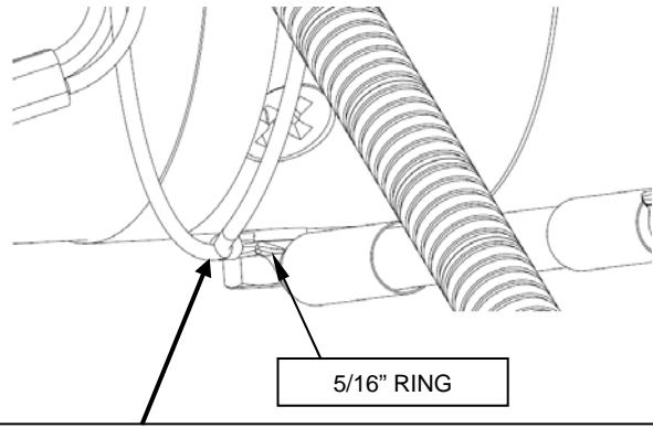
INSTALL BLACK WIRE WITH 5/16" RING UNDER 2 AWG GROUND CABLE TERMINAL. TORQUE NUT TO 75in-lbs (9Nm)
