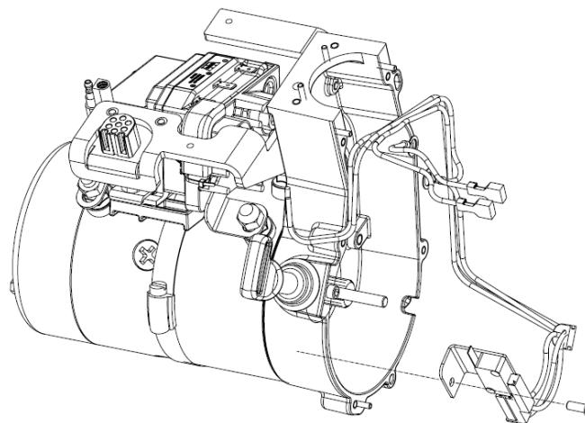
INSTALL WIRE HARNESS LIMIT SWITCH INSIDE CRANK CASE
