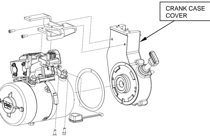
INSTALL RECEPTACLE CAP (ITEM #3) ON REMOTE RECEPTACLE. THEN ATTACH REMOTE RECEPTACLE TO COVER BRACKET (ITEM #2) TO CRANK CASE COVER WITH 10-24 HEX SOCKET SCREWS (ITEM #15).
