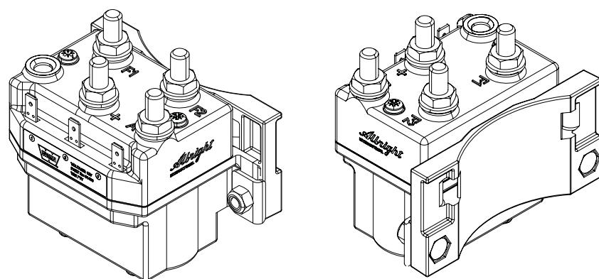
INSTALL (2) NUTS (ITEM #12), AND TORQUE TO 40 in-lbs (4.5Nm)
