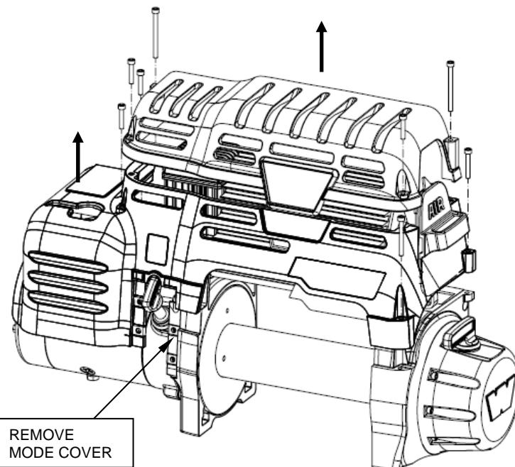
REMOVE HEX SOCKET SCREWS HOLDING TOP COVERS, AND MODE COVER BUTTON HEAD CAPSCREWS.
