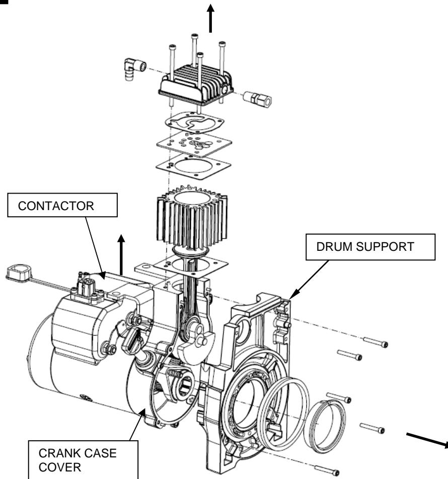
SEPARATE CRANKCASE COVER FROM DRUM SUPPORT. REMOVE CYLINDER HEAD. REMOVE MOTOR. REMOVE CONTACTOR. WHEN REMOVING MOTOR FROM THE CRANK CASE COVER APPLY PRESSURE TO MOTOR SHAFT SO THAT THE ARMATURE DOES NOT COME OUT OF MOTOR HOUSING OTHERWISE THE BRUSHES WILL NEED TO BE RESET.
