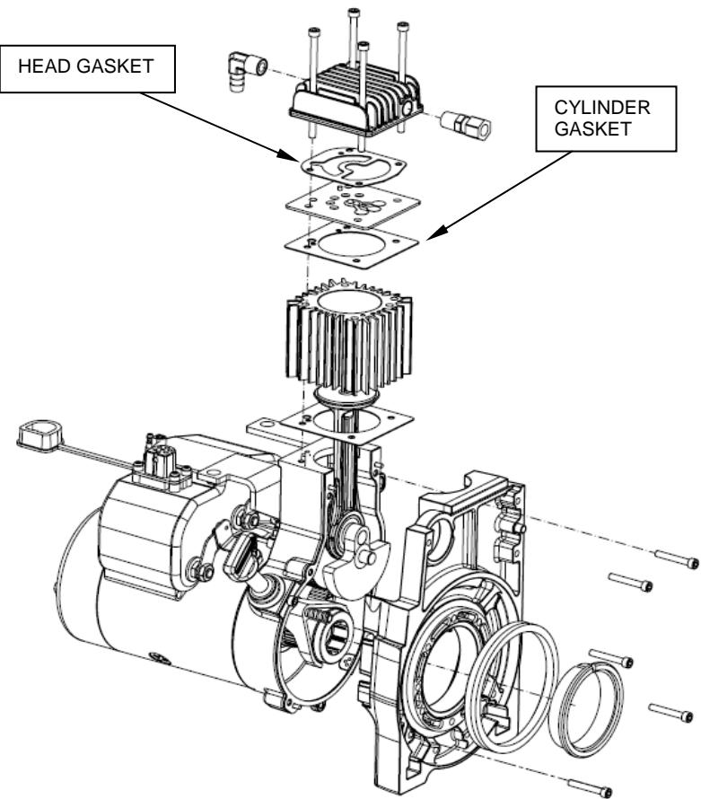
RE-ASSEMBLE CYLINDER HEAD. RE ASSEMBLE CRANK CASE USING NEW REPLACEMENT GASKETS (ITEM# 23 AND 24) AND ATTACH TO DRUM SUPPORT. ATTACH DRUM SUPPORT TO INTER COOLER WITH 3 10 inch LONG SOCKET HEAD SCREWS.
