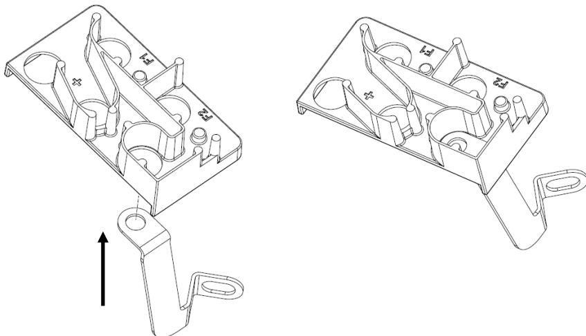
INSERT BUS BAR (ITEM #4) INTO SEPARATOR (ITEM #8) AS SHOWN
