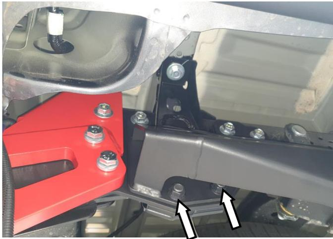
56. Fit the two M12x30 (8.8) flange bolts and flange nuts from the lower tube kit if there are no recovery points fitted.
