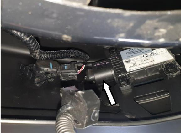
39. Connect the plugs to the radars. Ensure they are fully clipped in.
