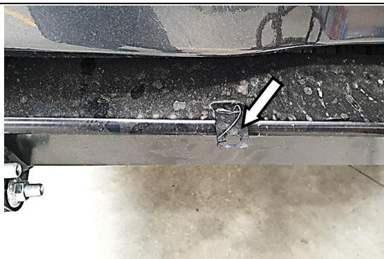
9. Using pliers, bend the LHS bracket up 90° as shown.
