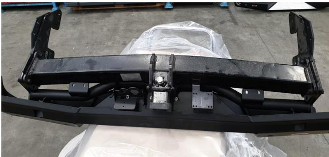
28. Loosely fit the Toyota tow bar and side mount plates in the ARB rear bar using the shims and bolts removed in step 11.
