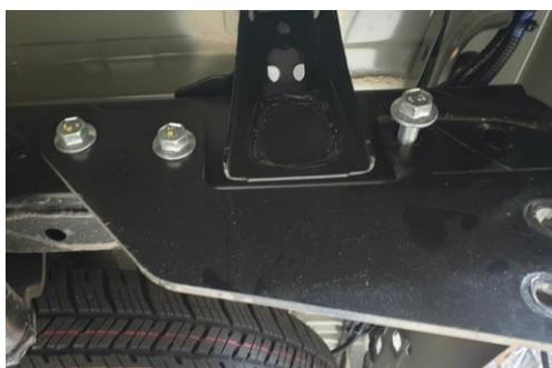
13. Remove the tow bar mount plates from the chassis by removing the three bolts per side. Set mount plates and bolts aside for refitment later.
