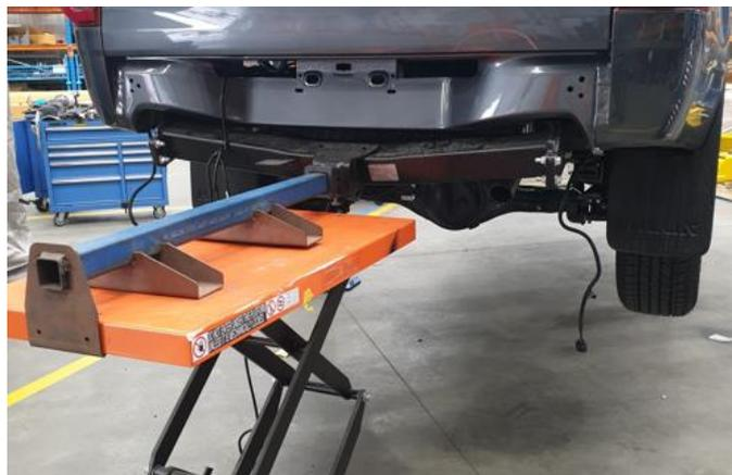
10. With the aid of a lifting trolley, support the tow bar so that it can be removed.
