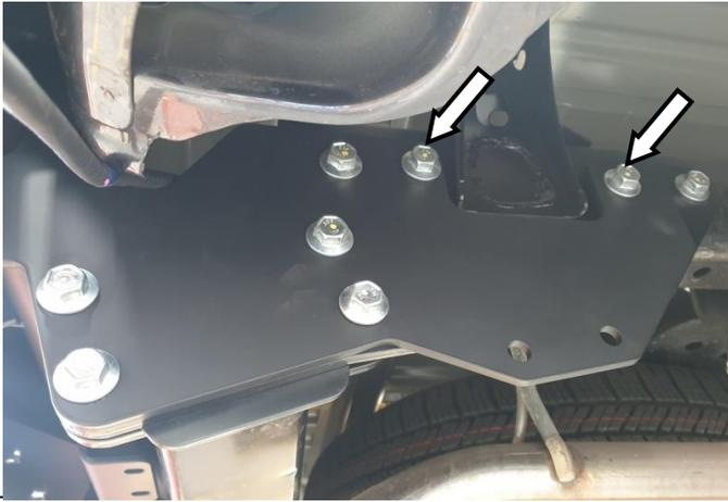
52. Remove the two M12 bolts per side shown and set aside for refitment later.
