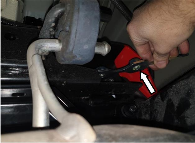
48. Feed the nut stick in through the rear of the chassis and line it up with the two mount holes.
