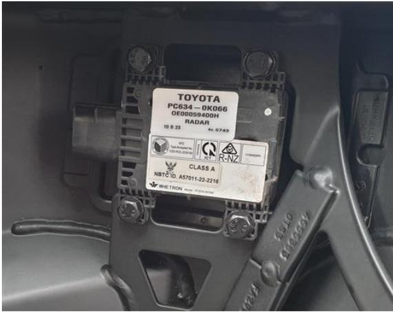
34. Install the radars removed in step 3 using four M6x20 bolts, washers and flange nuts per side.
