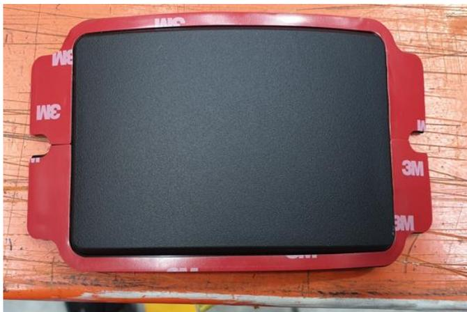
32. Fit the radar gaskets to the radar covers as shown.
