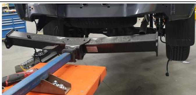
12. Remove the tow bar from the vehicle.
