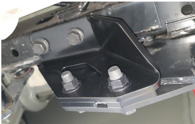
49. Loosely fit the support brackets to the inside of the rear bar using two M12x40mm flange bolts and flange nuts.
