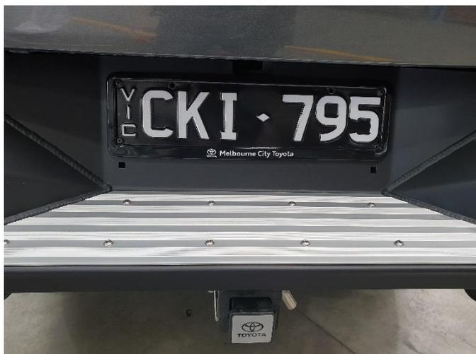
37. Fit the licence plate using four self-tapping screws.
