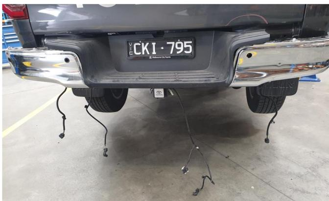
4. To remove the bumper from the vehicle, the parking sensors need to be removed and the wiring harness needs to be routed out of the way. (There is no plug to disconnect the harness).
