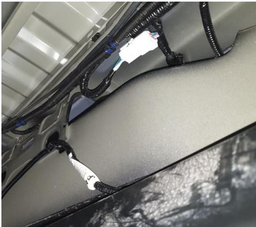
41. Using the cable ties provided, secure the wiring harness up out of the way, and keeping it free from the exhaust.
