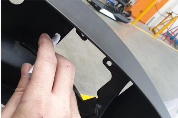
31. Use the supplied 3M primer stick on the inner face of the radar cut-out on the ARB bar as shown.
