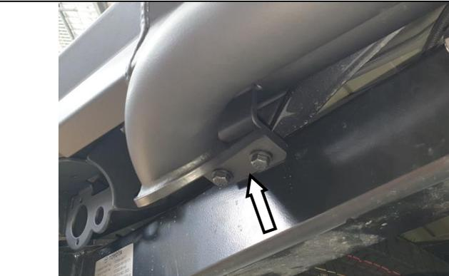
57. Fit two M8x25 bolts, washers and flange nuts to the inboard bracket on each tube assembly. Leave finger tight.
