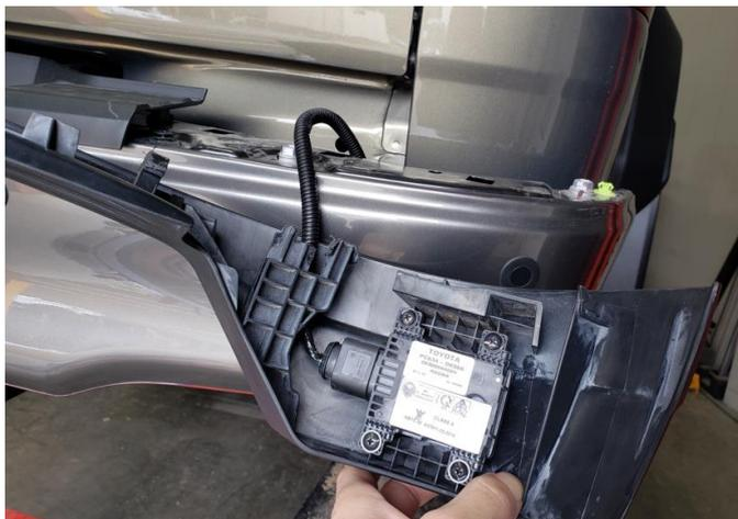
3. The radars need to be removed to disconnect the harness. Remove the 4 screws that retain each radar and then disconnect the radars.
