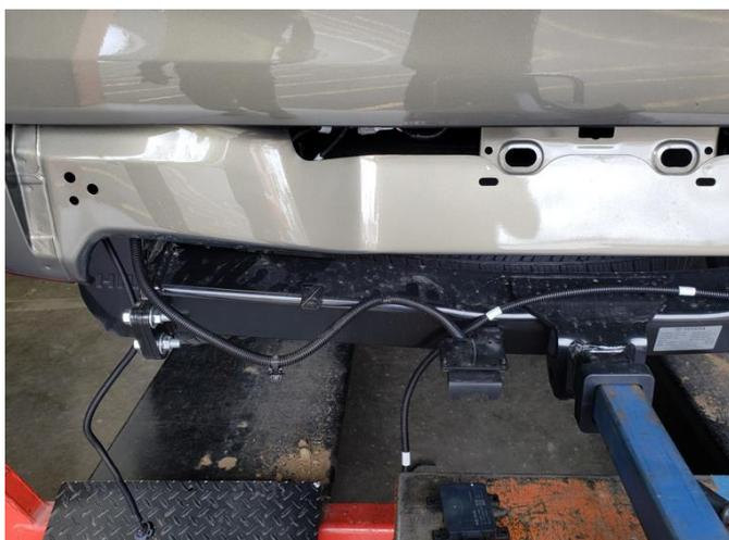
8. If the vehicle comes with a trailer plug, remove it and let it hang down with the rest of the loom. Set the fasteners aside for refitment later.
