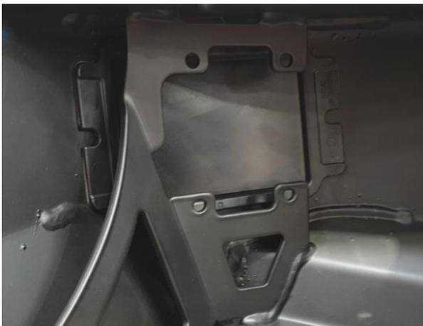
33. Fit the radar covers in the bar as shown. They must be firmly pushed into position.
