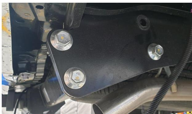
11. Remove the three bolts and two shims per side and set aside for refitment later.
