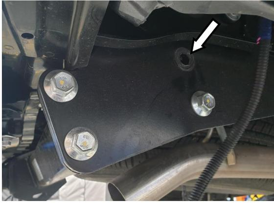
5. Remove the upper rear bolts on the tow bar and retain the bolts for re-fitment later.
