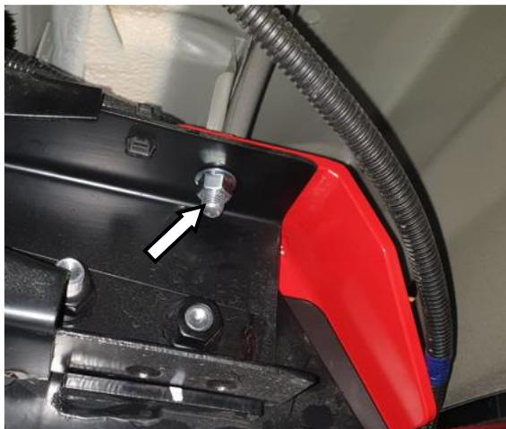
46. Fit one M10x30 bolt, washer and flange nut to the top hole of each recovery point as shown.
