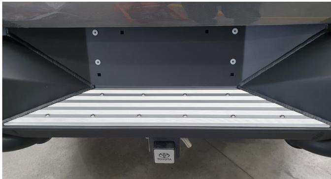
36. Fit the tread plate using ten M6x16mm stainless steel button head screws and stainless washers.
