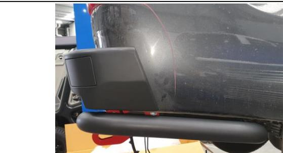
58. Adjust the tube so that it sits parallel to the vehicle tub as well as the ARB rear bar wing.
