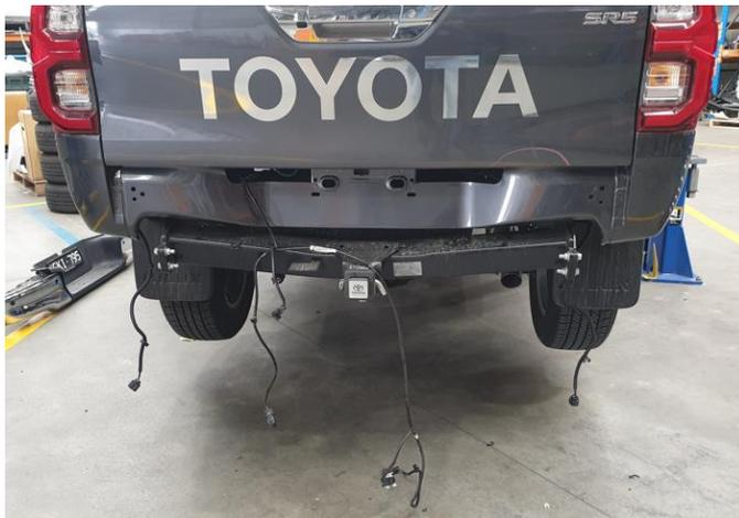
7. Remove the rear bumper and set aside. Carefully unclip the parking sensor housings from the bumper for fitment into the ARB rear bar.
