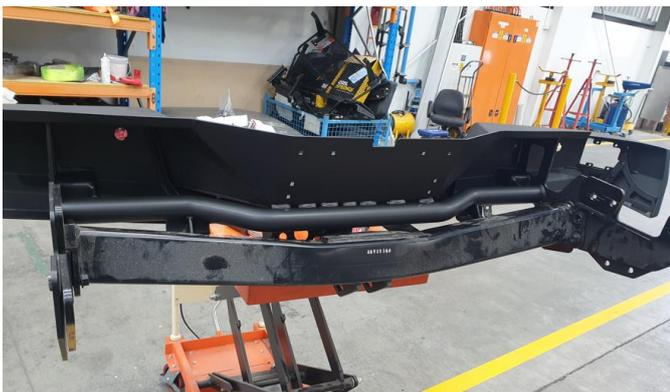
29. Support the rear bar on a lifting trolley as shown. Note the orientation of the tow bar and side mount plates in the image.
