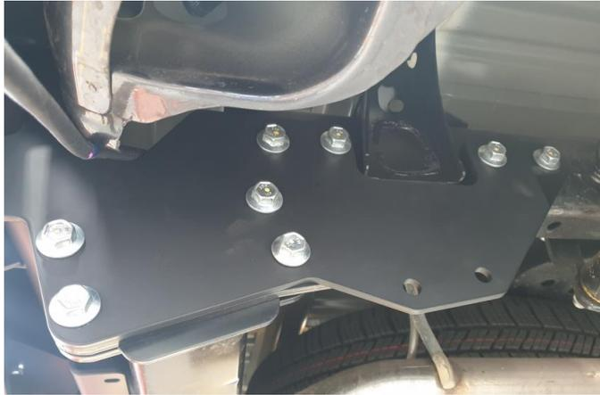
35. Offer the rear bar up to the vehicle and fit four M12 bolts per side removed from step 13.
